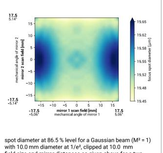
field size and mirror distances as given above for a two mirror scan system
